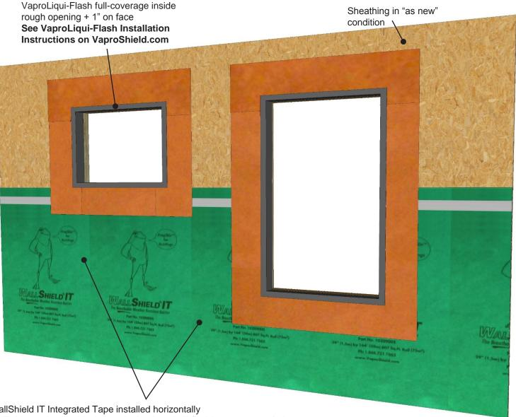
WallShield IT Integrated Tape installed horizontally
