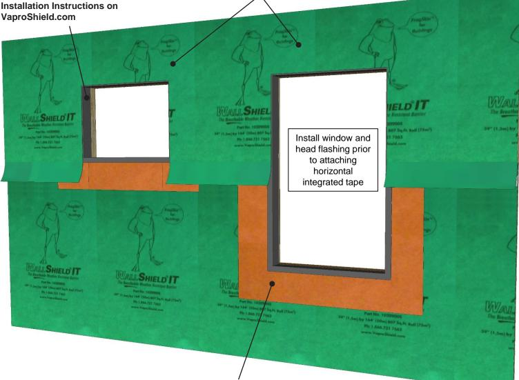
WrapFlashing SA properly shingled and folded 2.75" inside of R.O.
