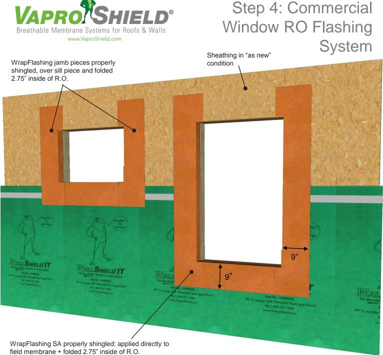
**Note**: Total of 11.75" of flashing should be used:
