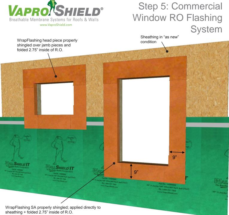
**Note**: Total of 11.75" of flashing should be used:
