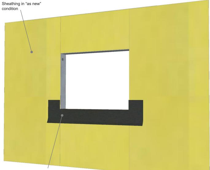
RevealFlashing SA Self-Adhered properly shingled; applied directly to sheathing + folded 2.75" inside of R.O. Note: Total of 11.75" of flashing should be used:
