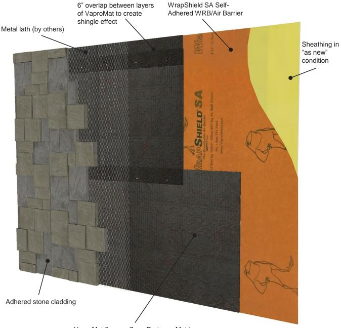
VaproMat 3mm or 7mm Drainage Matrix with attached filter fabric
