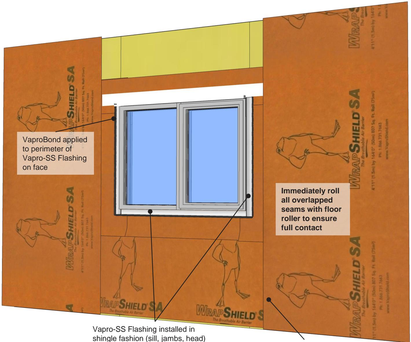
VaproBond applied to perimeter of Vapro-SS Flashing on face
