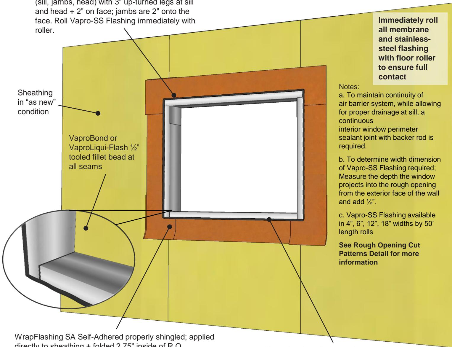
**Immediately roll all membrane and stainless-steel flashing with floor roller to ensure full contact**
