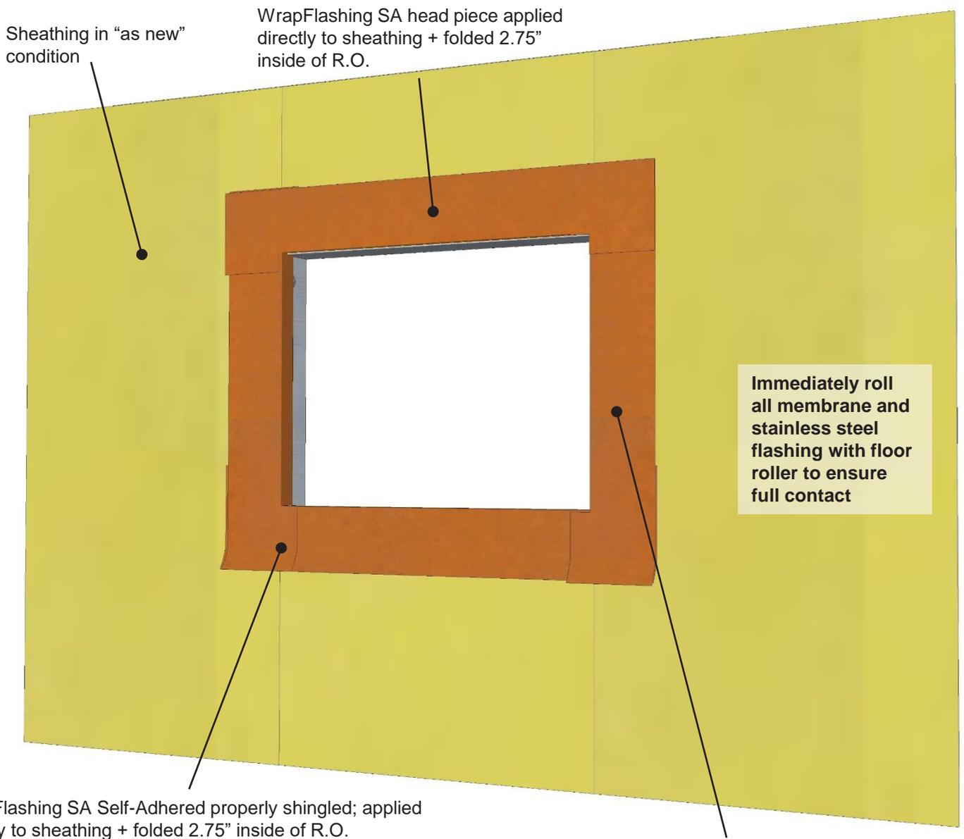
WrapFlashing SA Self-Adhered properly shingled; applied directly to sheathing + folded 2.75" inside of R.O.
