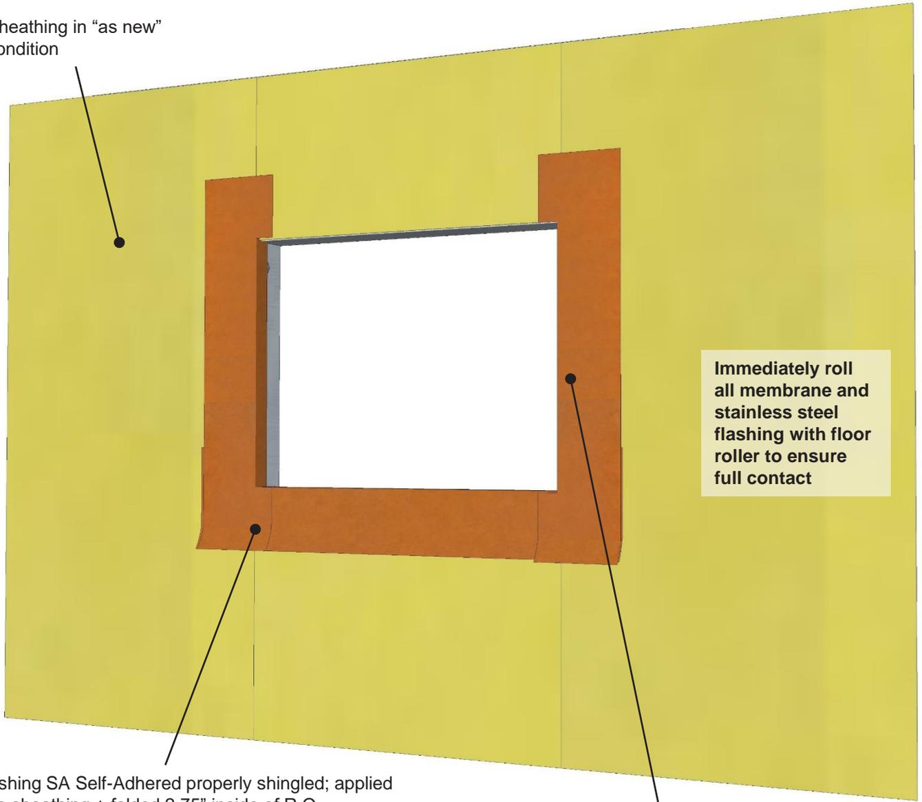
**Immediately roll all membrane and stainless steel flashing with floor roller to ensure full contact**
