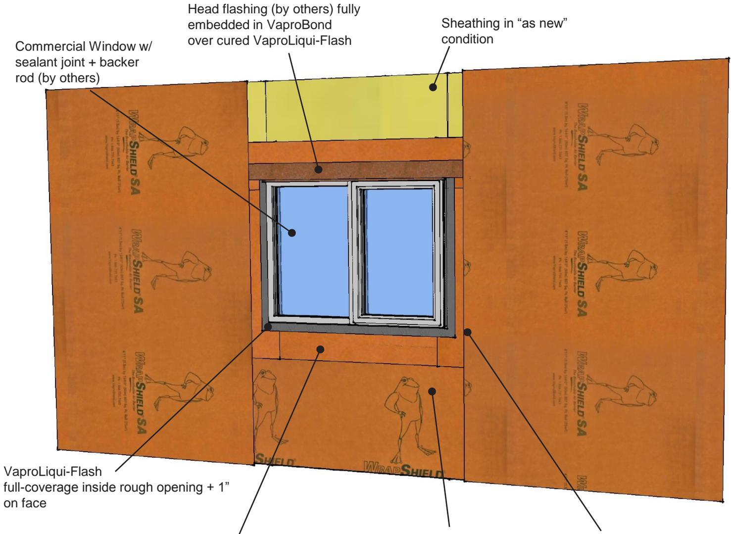
WrapFlashing SA Self-Adhered properly shingled; applied directly to sheathing + folded 2.75" inside of R.O.
