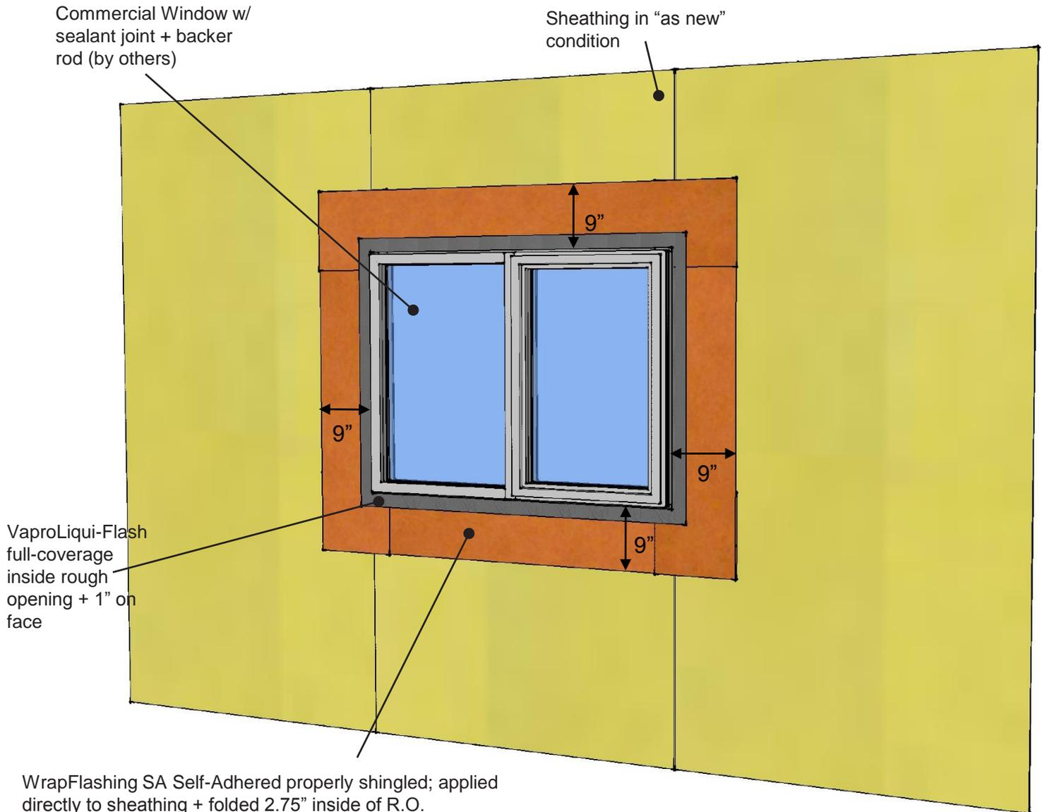
WrapFlashing SA Self-Adhered properly shingled; applied directly to sheathing + folded 2.75" inside of R.O.
