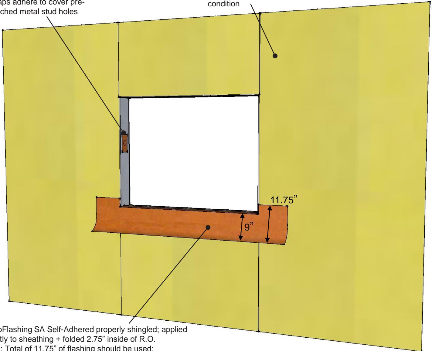
WrapFlashing SA Self-Adhered properly shingled; applied directly to sheathing + folded 2.75" inside of R.O.
