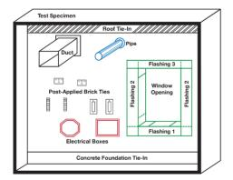
ASTM E2357 is a more realistic test method, emulating installed materials on a building
