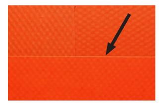
Figure 2, On the upper reverse lap seam, apply a bead of VaproBond<sup>™</sup> sealant the full length of the seam, as shown in Figure 3
