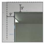
2. Measure and cut VaproFlashing SA sill, left & right jambs, and head flashing so that each piece extends 9" past edges of opening for each side (= R.O. + 18").
