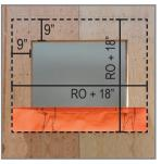
1. Measure and cut VaproFlashing sill, left & right jambs, and head pieces so that each piece extends 9" past edges of opening for each side (= R.O. + 18").
