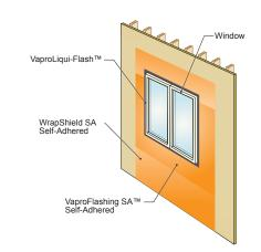
VaproShield's systems approach reduces contractor liability by using fully tested VaproLiqui-Flash and pre-cut VaproFlashing SA Self-Adhered to flash the rough openings.
