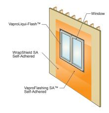
VaproShield's systems approach reduces contractor liability by using fully tested VaproLiqui-Flash and pre-cut VaproFlashing SA
