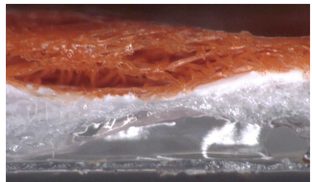
WrapShield SA Self-Adhered is a triple layer polypropylene micro-porous film laminate with a proprietary acrylic vapor permeable adhesive.
