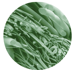
WallShield triple layer spun bond polypropylene.
