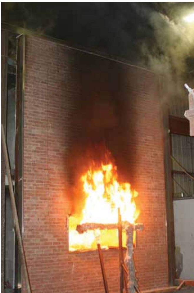
Figure 2. An NFPA 285 test in progress.
