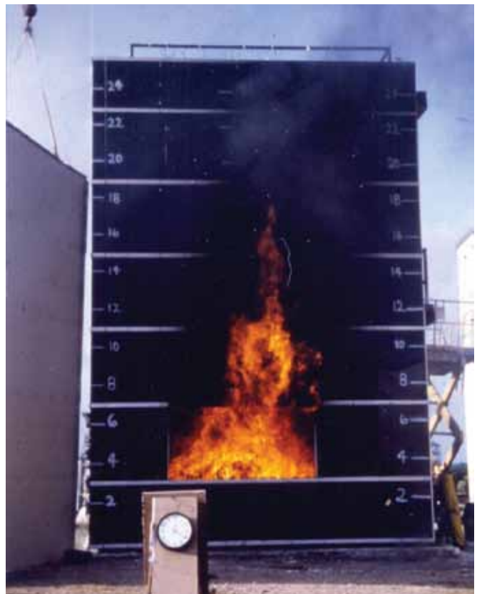
Figure 1. UBC 17-6 test in progress.
