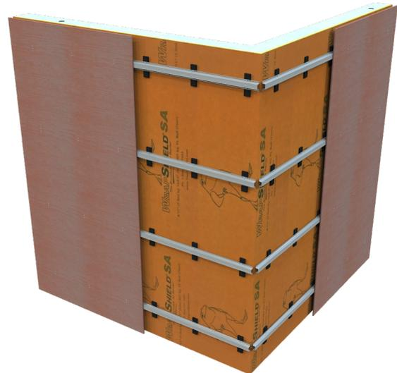
VaproShim SA adheres to vertical hat channels, sealing fastener penetrations and creating a vertical rain screen drainage plane, adding significant drying capacity to building envelope.
