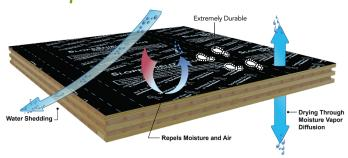
A In a drying study, conducted by RDH Building Science Laboratories, SlopeShield Plus SA allowed a wet (42% moisture content) mass timber panel to dry to below 20% moisture content in 14 days.
