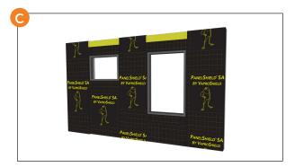
As the wall substrate is erected install a VaproShield continuous vapor permeable air barrier to protect walls and rough openings.
