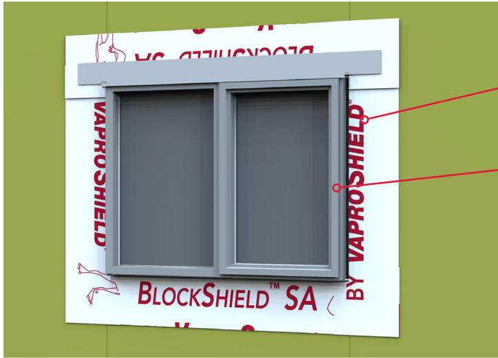
BlockFlashing properly shingled and applied directly to the sheathing
