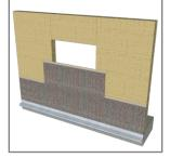
4.Install cut piece over window rough opening leaving 12" each side.
