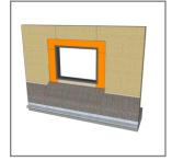
9. Install VaproLiqui-Flash in rough opening as shown. (View VaproLiqui-Flash details at VaproShield.com).
