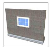
17. Install next horizontal course of RSSA over headflashing. Notch and trim if required to fit.
