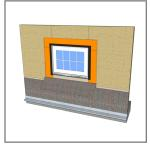
11. After window installation, seal nail flanges at jambs and head with VaproLiqui-Flash or VaproTape.
