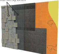
9. Apply thin-set stone according to manufacturers' recommendations. Guidelines should include a weep method for ventilation and drainage as recommended.
