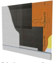
9. Apply stucco according to manufacturers' recommendations. Guidelines should include a weep method for ventilation and drainage as recommended by Northwest Wall and Ceiling Bureau details www.nwcb.org.
