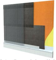
8. Install expanded metal lath over the VaproMat according to the manufacturers' recommendations. Consult NW Wall and Ceiling Bureau, nwcb.org, for details regarding drainage stucco systems. All lath including weep screeds are installed "proud" or over the VaproMat material.
