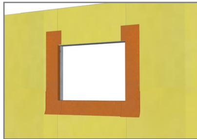
2. Install jamb pieces with 2.75" (70 mm) folded into R.O. 9" (229 mm) to be left on face.
