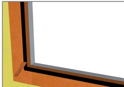
5. Immediately spread the applied material with a putty knife creating a 1" (25 mm) border around the rough opening.
