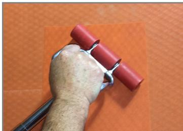
Use hand roller to ensure complete adhesion.
