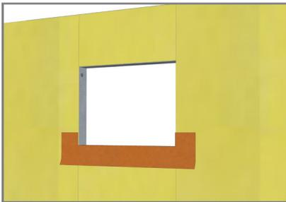
1. Install VaproFlashing SA Self-Adhered (orange) or RevealFlashing SA (black) into sill with 2.75" (70 mm) folded into Rough Opening (R.O.) 9" (229 mm) left on face, with bottom 6" (152 mm) of release film to remain
