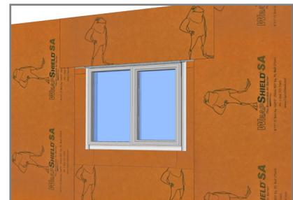
9. Install WrapShield SA field membrane over metal head flashing, maintaining 3" minimum overlap to adjacent field membrane. roll to ensure adhesion at seams (overlaps).
