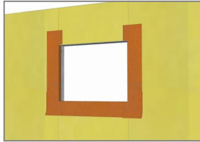
2. Install jamb pieces with 2.75" folded into R.O. 9" to be left on face.
