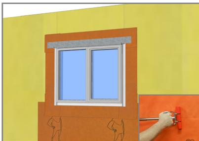
7. Install field membrane underneath 6" flap of sill flashing to create shingle effect, remove release film, adhere to membrane, roll to ensure adhesion at seams (overlaps).
