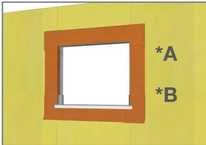
4. Install Vapro-SS Flashing at sill in shingle fashion with 3" up-turned legs at sill and head + 1" on face; jambs are 1" onto the face.
