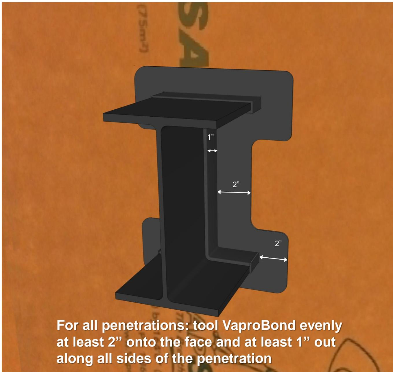
**For all penetrations: tool VaproBond evenly at least 2" onto the face and at least 1" out along all sides of the penetration**
