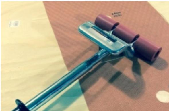
*Figure 1, Ensure the reversed lapped WrapShield SA Self-Adhered is bonded to the surface by utilizing a hand roller such as the Superior-Hand-Roller-80-R32-M.*
