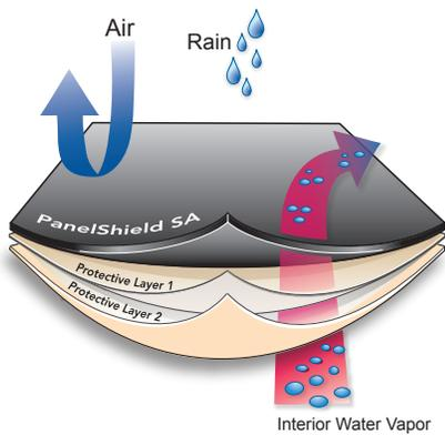
An enemy of any home is air leakage and moisture infiltration. Similar to Gore-Tex®, VaproShield membranes stop air leakage provide exceptional water holdout and breathability, mitigating mold and reducing energy costs for the life of the home.
