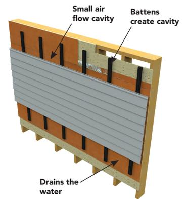
Installing a drainage matrix, battens, or shims, leaves a small air flow cavity behind the cladding, allowing residual water to drain away from your home. Plus, water vapor passing from the inside to the outside can diffuse through the air cavity. The practice is called rain screen design, it's a proven method to keep the wall assembly dry.
