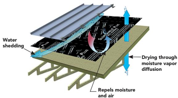
SlopeShield Plus SA vapor permeable air barrier roofing underlayment blocks air infiltration yet allows moisture to flow through and evaporate, instead of remaining trapped in the roofing materials. It can be used together with ice and water shield.
