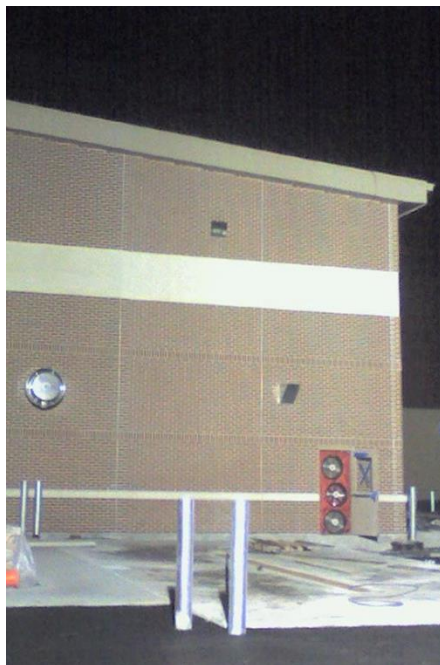
Figure 4: A “blower door” installation fitted to the exterior doorway for a USACE air barrier pressure test.
