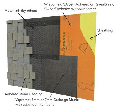
VaproMat's lightweight filter fabric is designed to keep the drainage cavity clean and unobstructed during the lath/plaster, or adhesive mortar installation. VaproMat promotes rapid drying along with stability to the polypropylene matrix.
