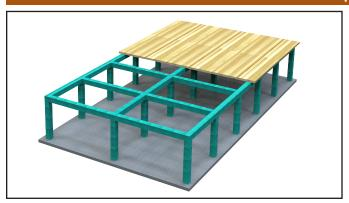
5. Construct mass timber floor/deck. Remove top pieces of Wallshield IT just before panels are laid.
