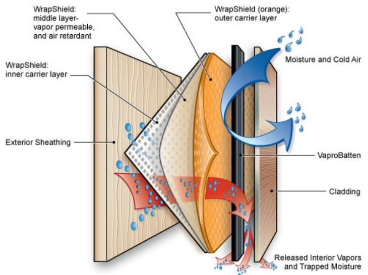
*A mechanically attached, water resistive, vapor permeable air barrier membrane, WrapShield features integrated tape at the horizontal seams to dramatically reduce installation time and material expenses.*
