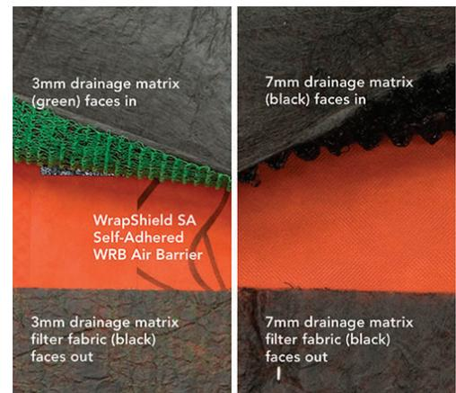
*VaproMat, installed over VaproShield membranes, creates a positive drainage cavity. Ideal for use behind stucco, stone, and traditional cladding systems. The filter backing keeps the drainage cavity clean during lath and plaster.*
