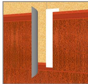
6. Install WrapShield RS abutting piece with joint centered on WrapFlashing SA. Use hand pressure to engage the pressure sensitive adhesive.
