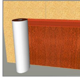
2. At the base of the wall, begin installation with SS staples in the top 2" above the tape. Snap a line for guidance. **Do not staple in the tape area.**
