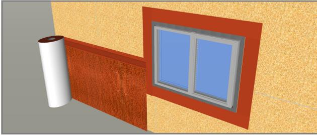
1. Flash all window and door rough openings with VaproLiqui-Flash and WrapFlashing SA prior to WrapShield RS Rain Screen field material installation. Refer to the following documents at [www.VaproShield.com](http://www.VaproShield.com):
