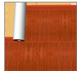
11. Secure material to substrate using only recommended gasketed fasteners in the field area of WrapShield RS, as previously noted in this document. Continue up the wall in shingle fashion. Repeat as needed.
