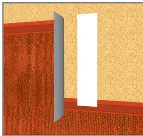
4. Staple 1 1/4" WrapFlashing SA Self-Adhered, centered behind vertical joint location, with white adhesive side out. Lap over lower course, halfway onto tape joint [approx. 3.5"], as shown. Place butted joint at middle of WrapFlashing SA Self-Adhered.
