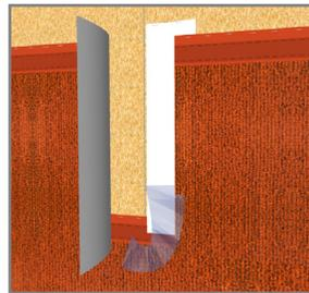
5. Remove release film of WrapFlashing SA Self-Adhered. Note: mechanically attached WrapFlashing SA may be used in lieu of WrapFlashing SA, with a 3/8" bead of VaproBond Adhesive Sealant, blind sealing behind each flap.
