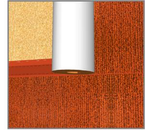
3. Line up the bottom of the upper course of material with the dotted line, creating a 6" overlap, progressing in a shingle fashion up the wall.
