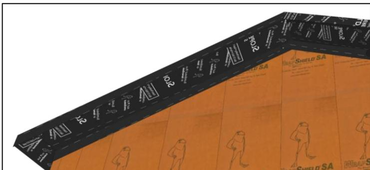
If desired adhesion is not attained between membranes due to site conditions, VaproShield recommends applying a bead of VaproBond as an additional solution to pressure rolling.
