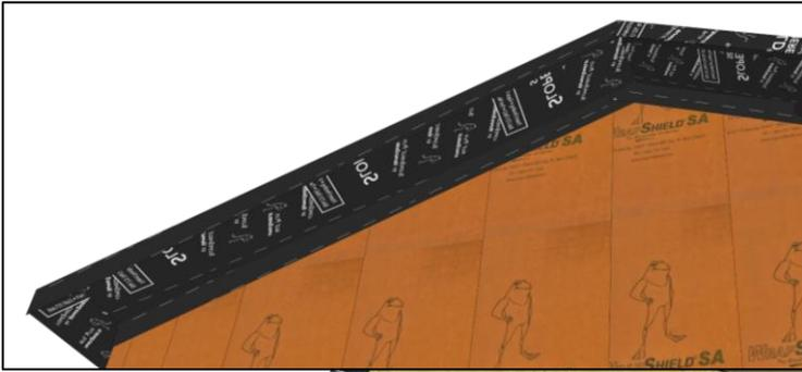
If desired adhesion is not attained between membranes due to site conditions, VaproShield recommends applying a bead of VaproBond as an additional solution to pressure rolling.
