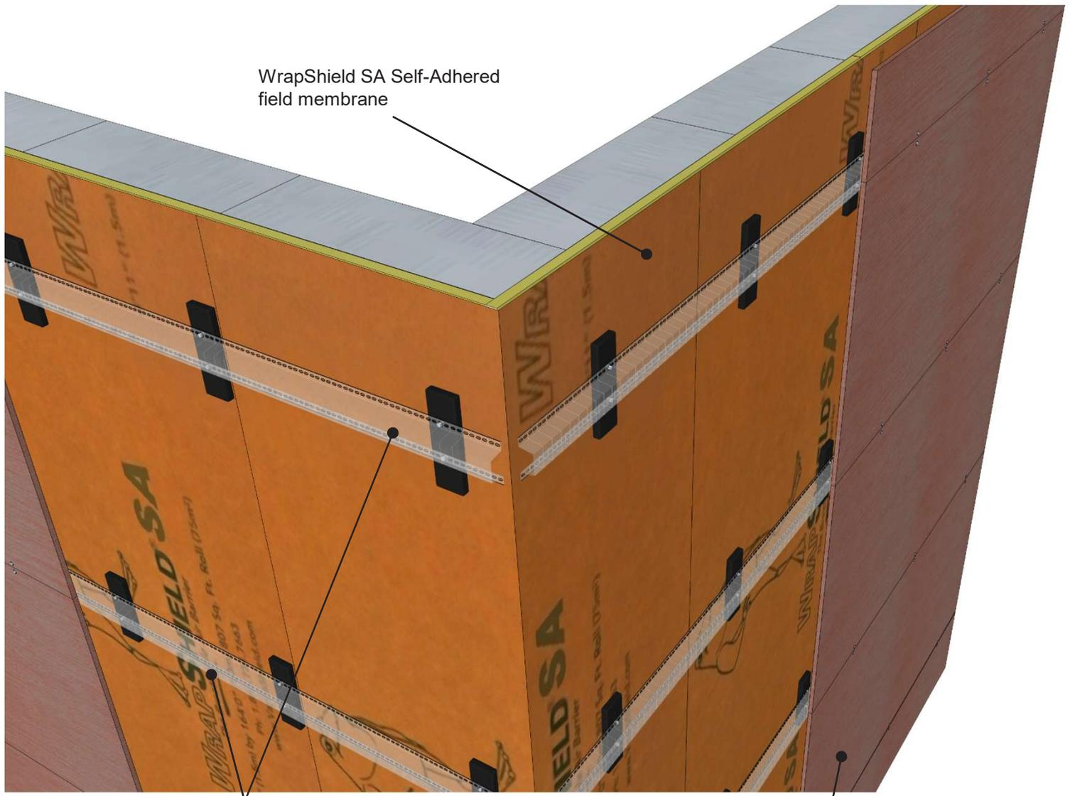
WrapShield SA Self-Adhered field membrane
