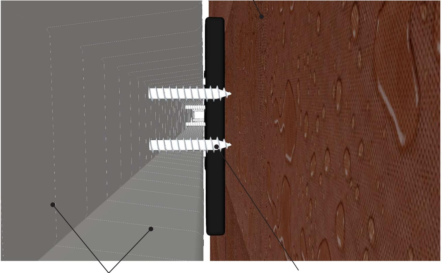
Horizontal hat channels screwed into VaproShim SA Self-Adhered, creating a drainage gap between cladding attachment system and field membrane
